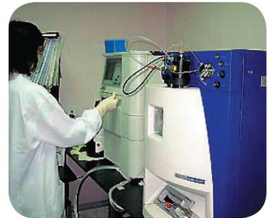
■ 篩檢儀器—串聯質譜儀 ( Tandem Mass Spectrometry )
